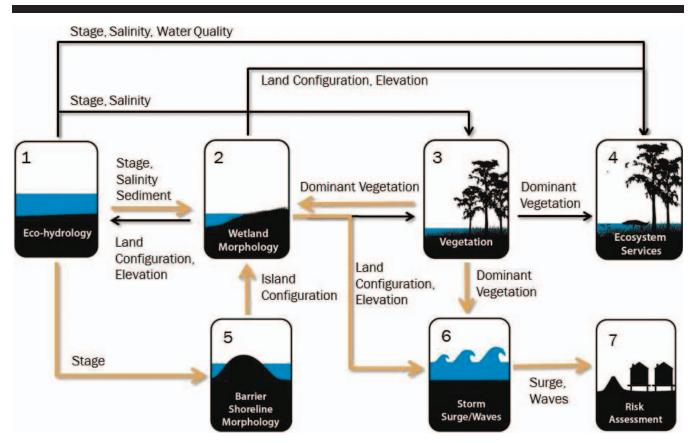
Figure 3. The modeling framework for the 2012 Coastal Master Plan used a series of integrated, coastwide predictive models within a systems context (CPRA, 2012, Appendix D). The main input and outputs of each model that are linked to other models are indicated. The yellow arrows indicate substantially improved or entirely new feedback and links developed and utilized to support the 2012 Coastal Master Plan process.
