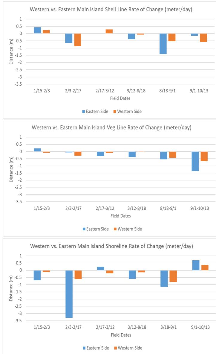
Figure 18: Graphs showing rate of change for shoreline, shell line, and vegetation line (m/day). Lines previously defined. Negative values represent retreat/movement towards interior of island and positive values represent advancement/seaward movement. Eastern side is defined as transects 4-10 and the western side 1-3 and 11-13. Main island only.
