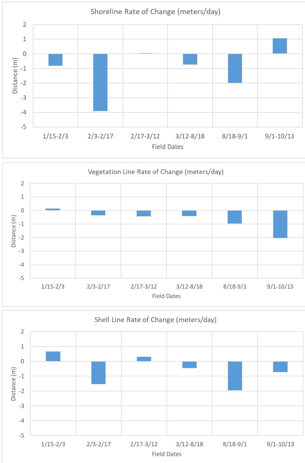
Figure 17: Graphs showing rate of change for shoreline, shell line, and vegetation line (m/day). Lines previously defined. Negative values represent retreat/movement towards interior of island and positive values represent advancement/seaward movement.
