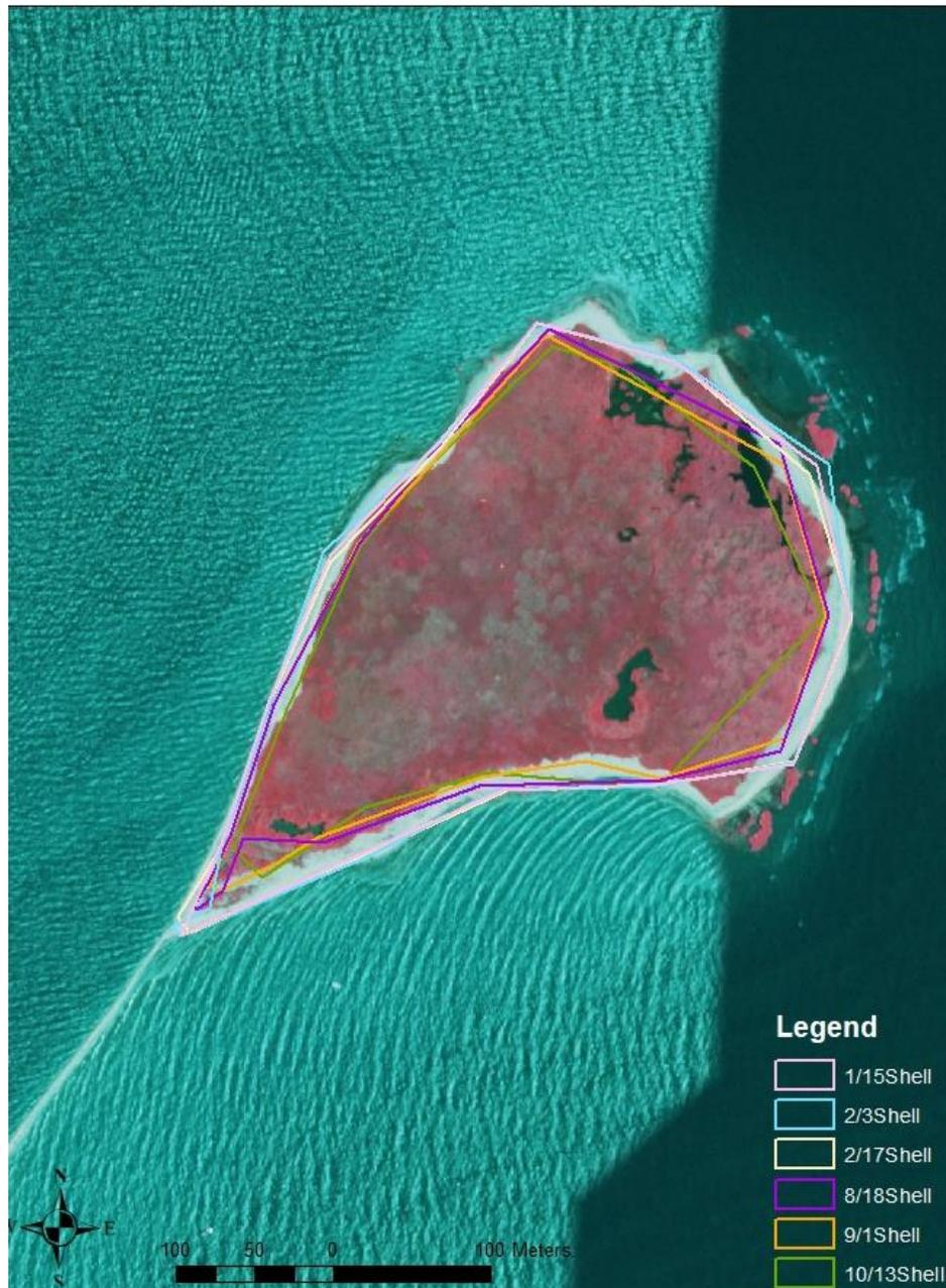
Figure 15: ArcGIS image showing the shell line polygon for all data sets except 3/12. The data is overlaid on NAIP 2019 imagery.
