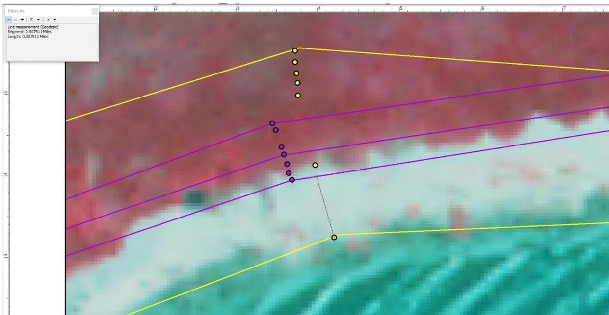
Figure 8: Zoomed in image of transect 6 with September 1 data shown in purple and October 13 data shown in yellow. The grey line represents the line created by using ArcGIS's measure tool. This shows the water line 'advancing' seaward from Sept 1 to Oct 13.
