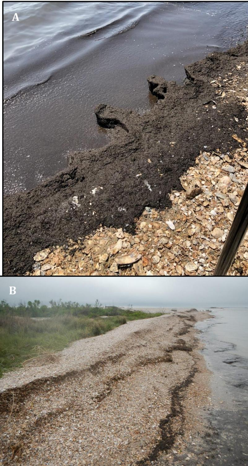
Figure 20: In between transect 2 and 3 on 3/12/2020 for image B and 8/18/2020 for image A. Image A shows the marsh platform at the water's edge eroding due to wave activity. The marsh platform is a sawdust consistency in the water. Image B shows the bigger picture of the area to show the shoreline's morphology.
