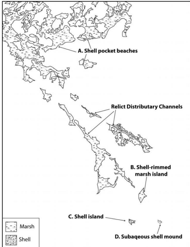
Figure 22: Plan-view conceptual geomorphic model from Ellison (2011). Model suggests a progression of shell pocket beaches to subaqueous shell mounds. Relict distributary channels are preferentially preserved due to their lithology being more resistant to erosion. As the channels become isolated, shell rimmed islands form and eventually become shell islands due to their inability to vertically accrete. Eventually, the entire mass submerges to a subaqueous shell mound.
