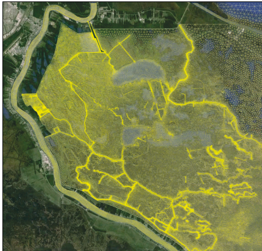
Figure 2-2. AOI inset mesh showing mesh elements (image courtesy Google).
