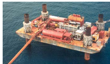
Complex pump arrangements, like the one on this sea-based platform, are often required to move slurry carrying particles of varied sizes over long distances.
