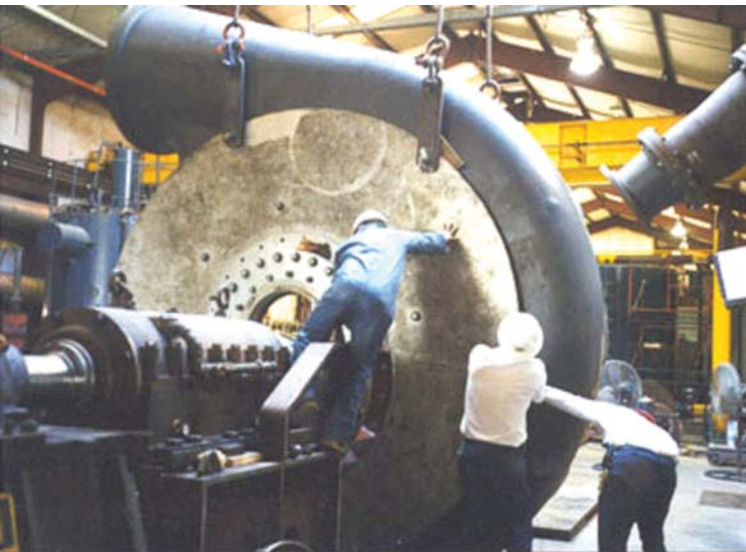
Centrifugal pumps on the dredge vessel and boosters every two to four miles along the pipeline keep the slurry moving. Longer pipelines require more pumps, increasing project cost.
