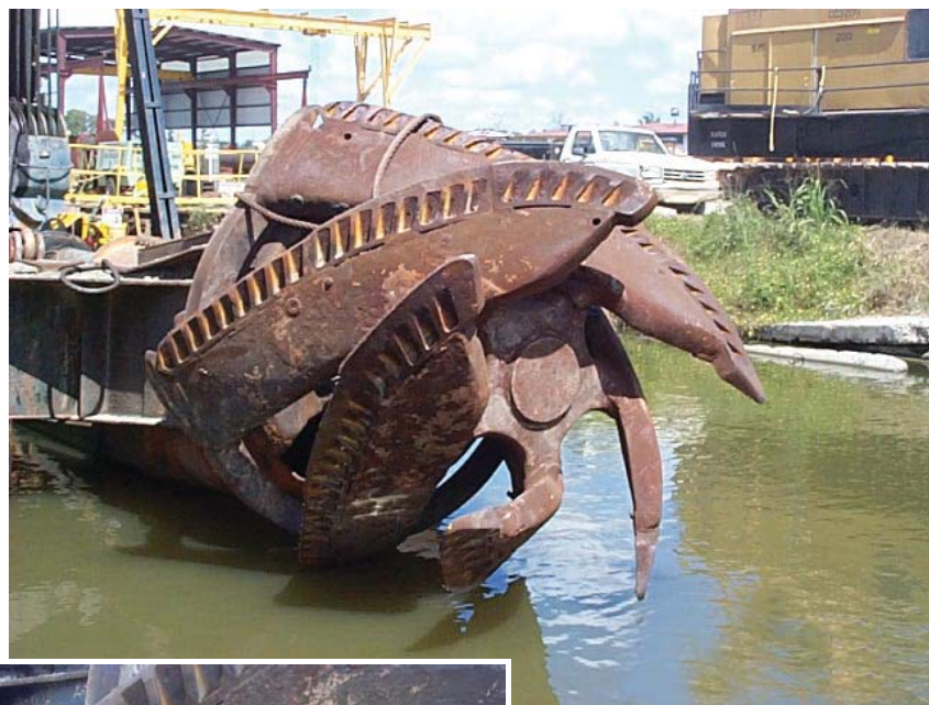
Above: The suction pipe on a pipeline dredge vessel is often fitted with a cutterhead, a massive mouthpiece eight or nine feet in diameter.
