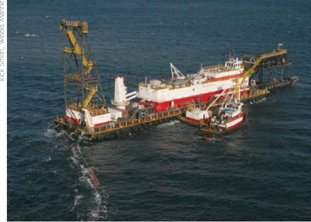
In coastal Louisiana, wetland restoration projects have typically used the pipeline dredge, a vessel specially designed to collect sediment and send it through a pipeline to the placement site.
